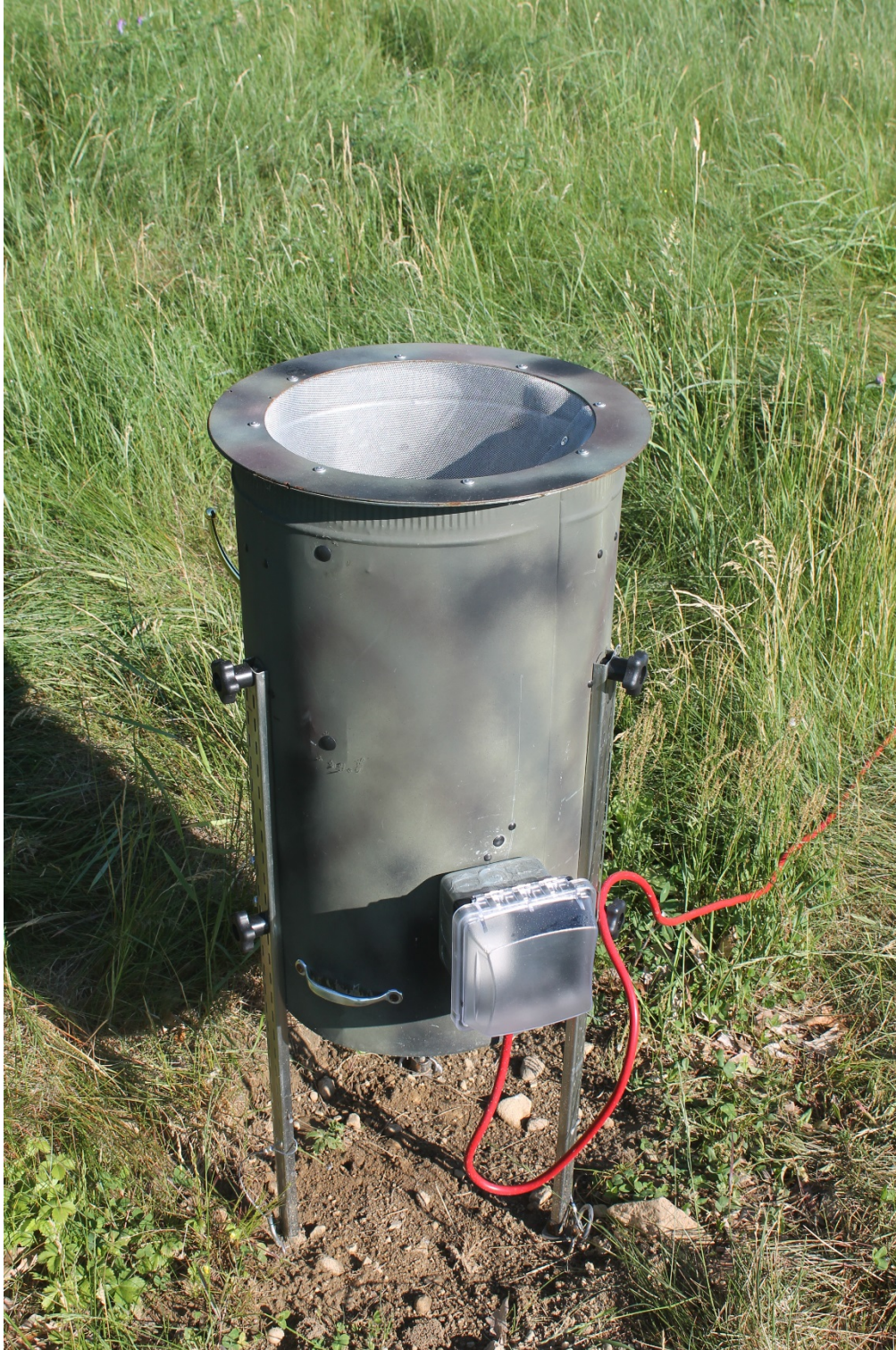
Figure A1. Modified Rothamsted-style suction trap used to collect daily samples of aerial insects (see also Macauley et al. 1988).
